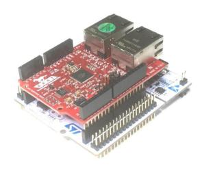
Fig. 5 The EasyCAT Shield on an STM32 NUCLEO board
